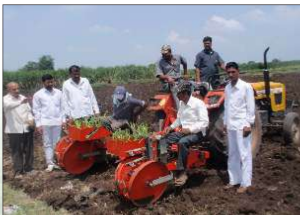
Sugarcane settling transplanting by using mechanical trasplanter
